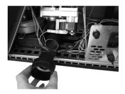
Fig. 38 - Remove the silicone fitting
