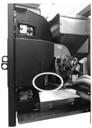
Fig. 51 - Remove screw 2
