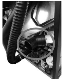
Fig. 30 - Position fitting at 45°
