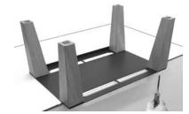
Fig. 12 - Fasten legs to the base
