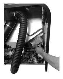
Fig. 29 - Fix the casing + fan to the stove
