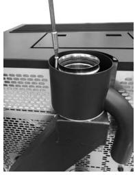
Fig. 37 - Secure the concentric pipe
